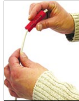
2 Slide Shrink Tube Sleeve Over Wire, Cable, Tube Or Round Object
